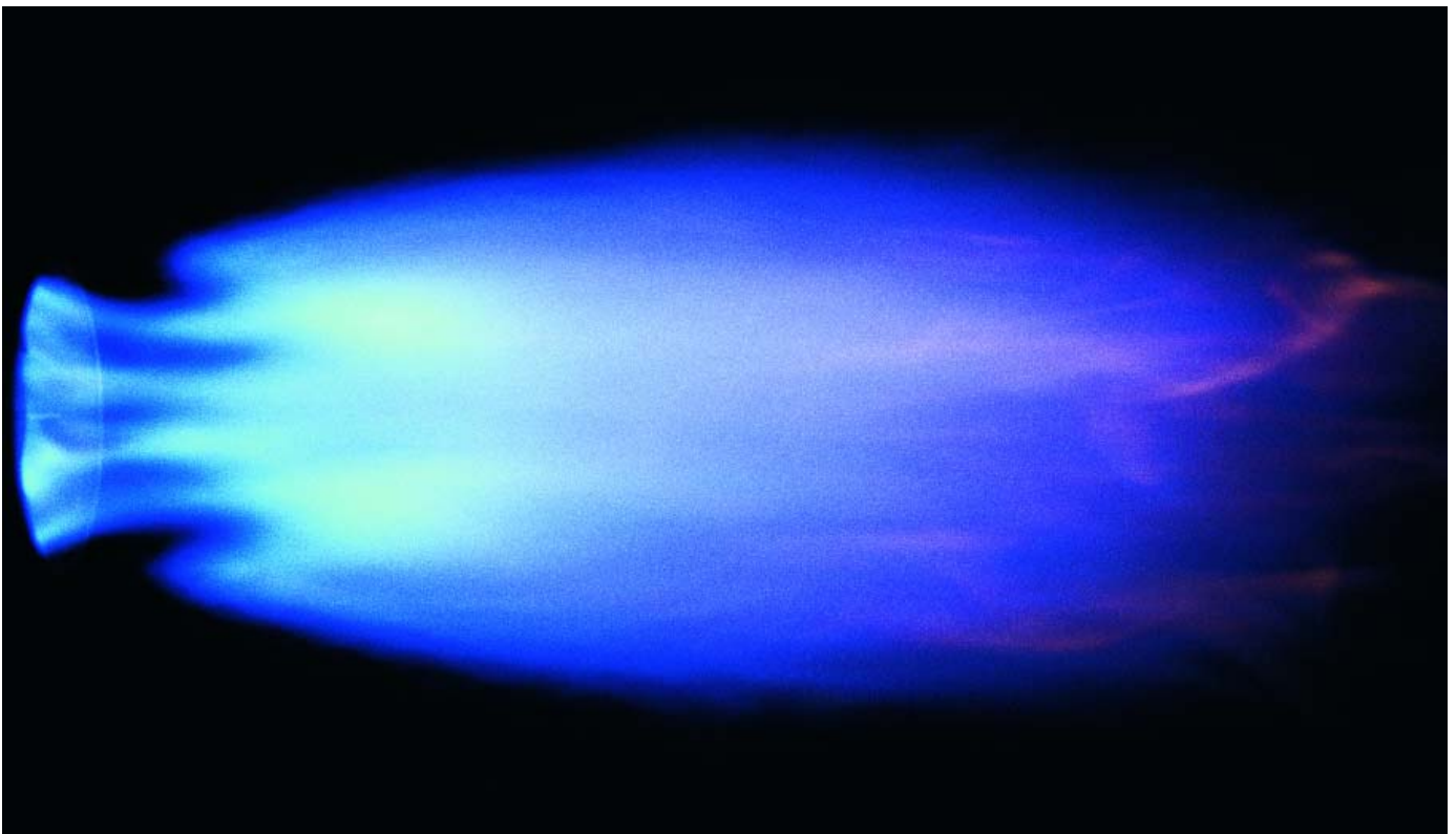
Typical flame formation for LN (LowNO x ) version gas burners
